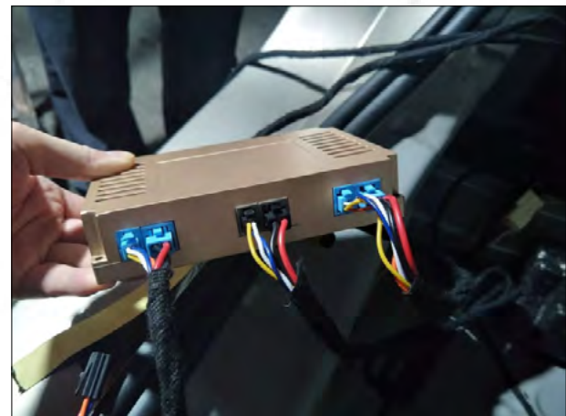
23. Insert the Hall line socket, the power cable socket and the electric suction lock cable socket into the control box, according to the color.
