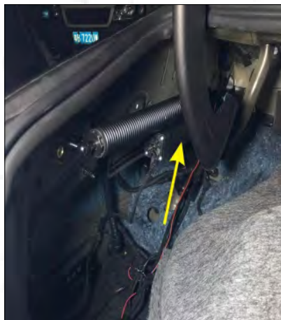
10. Install our left brace rod and the brace rod motor is facing the cab.
