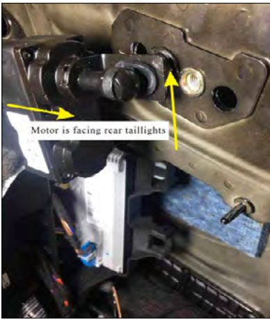
11. Install the ball head as shown by the arrow, the right side of the brace rod motor towards the rear taillights.
