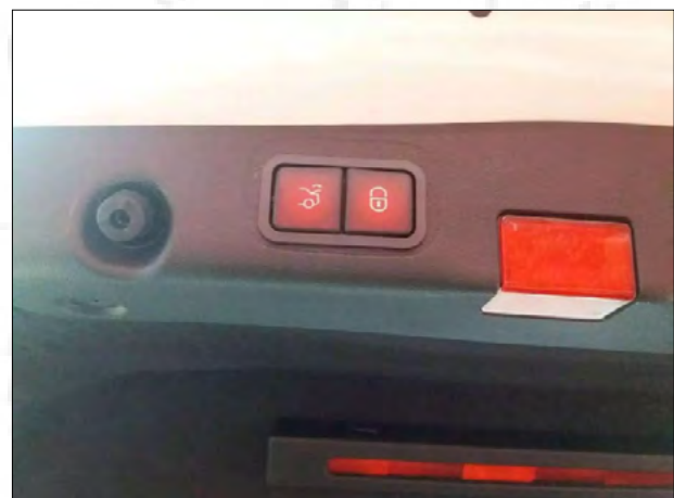
25. Install the tailgate switch button.
