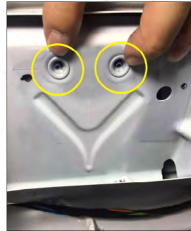
14. Remove the original car lock frame, as shown in the figure, our electric suction lock frame is installed at the position of the yellow circle.
