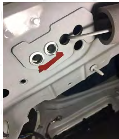
6. Put a rivet on the red mark hole on the left side of the trunk (The left and right steps are the same).
